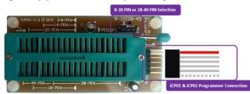
(this ZIF is easy to configure and use with just about ANY size thru-hole PIC, and any PICKit that supports ICSP capability. This is the ZIF the author uses for situations where there is no ICSP connector available. It is easy to use and very flexible.)
