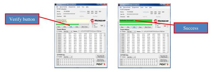
Once it verifies, your firmware is on the chip and you can disconnect the programmer (or remove it from the ZIF socket and install back in the board) and fire up the board to test.
